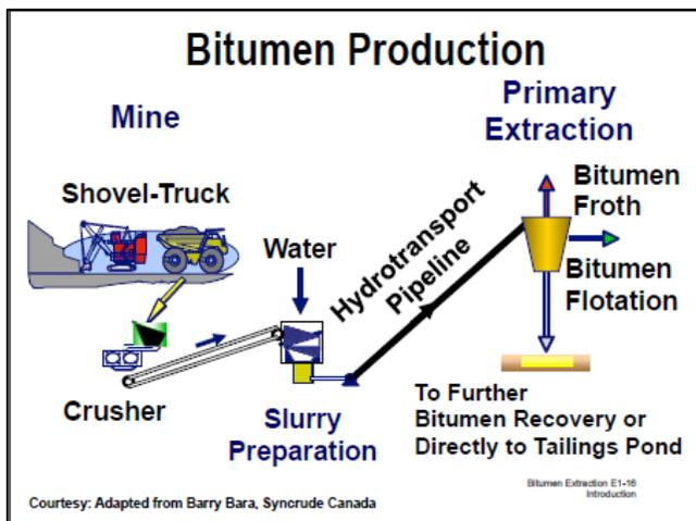
Typical Bitumen Production Process Schematic
